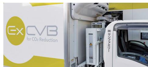
車載状態のバッテリー Swapping battery pack (between carburetor and accessories) at battery-swapping station
