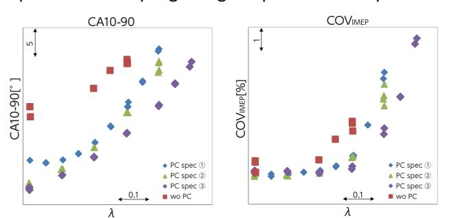
**Pre-Chamber Specification** 18 nozzles, small volume 210 nozzles, small volume 310 nozzles, large volume
