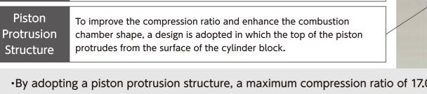
•By adopting a piston protrusion structure, a maximum compression ratio of 17.0 is achieved. •By modifying the pre-chamber fastening method and implementing a structure that allows the pre-chamber nozzle direction to be adjusted arbitrarily, heat loss from the walls is reduced and auto ignition in unburned regions is suppressed.
